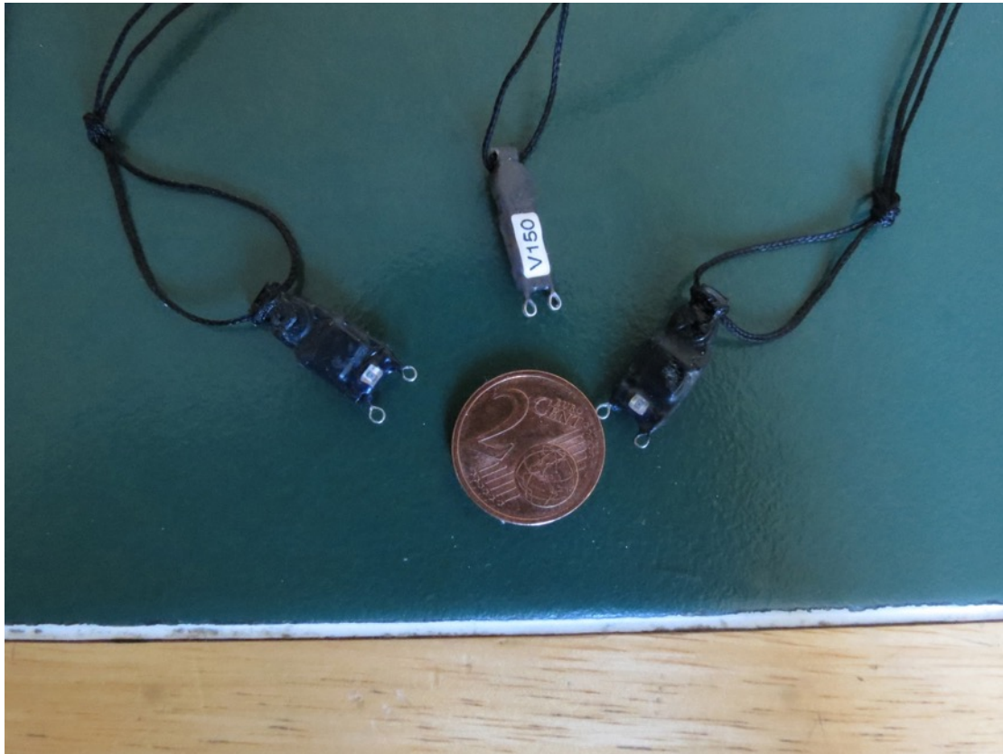
Photo 4: Geolocators: These tiny lightweight devices are being used to track a wide range of species on migration. 4 out of 7 fitted to Irish Swifts in Antrim and Tubbercurry last year are now being analysed to see where they, and the Swifts that carried them, have been for the winter. The wintering sites of Irish Swifts is believed to be in southern Africa but is not known .....yet!
