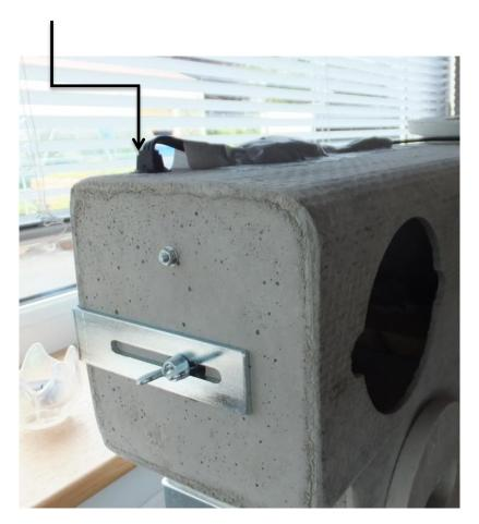
7. Finally stick the cabling to the box (ensure the place where the RCA connectors join is well covered) with duct tape to protect it from the weather.
