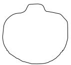
The size of this hole is very important because if it is too small the cables will not pass through, but if it is too big the junction box will not fit tightly. It is worth taking care over this.
